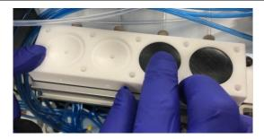
16. Reinstall the Top Manifold and screws. Make sure the manifolds are properly aligned to each other and the screw holes in the mounting bracket.
