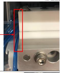
21. Verify that the two nuts on the air cylinder are both tight against the bracket.
