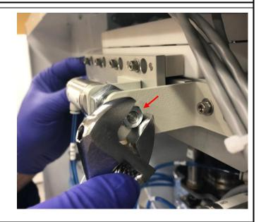
12. Slide the Connector plate to the left to remove it from the instrument.
