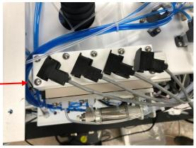
Lift the Top Manifold up and place it to the side.
