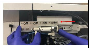
13. Inspect the Slide Bar for residue. If residue is present, clean the bar using a paper towel dampened with distilled water. Wipe until clean. Do not use any sharp objects which may damage the seals.
