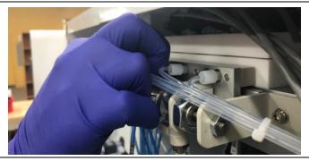
23. Loosen the four screws on the Connector plate until the gap reappears between the plate and the Slide Bar. The washer on the screw should be able to move freely once loosened.
