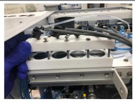
17. Tighten the screws in the following numbered pattern until they just contact the manifold (finger tight). Repeat the pattern (2) more times turning the screws 1/8 turn each time.
