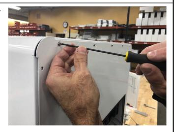
6. Slide the Nitrogen fitting out of the slot in the Rear Panel and remove the panel from the Instrument.
