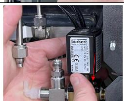
15. Using the 9/16" wrench, reattach the nut to secure the black cap in place.
