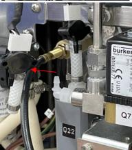
5. Using a 9/16" or adjustable wrench, loosen the nut holding the vent tube to the vent valve. Once loose, pull the vent tube up and out of its socket. Move to the side.
