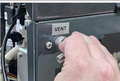
14. Reattach the black cap onto the vent valve.
