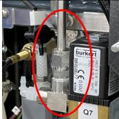
17. Reinstall the pressure sensor tube onto the valve by pushing the tubing back into position on the plug.
