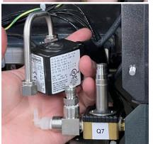
8. Using the 9/16" or an adjustable wrench, remove the vent valve outlet from the outer side of the DELTA cabinet.
