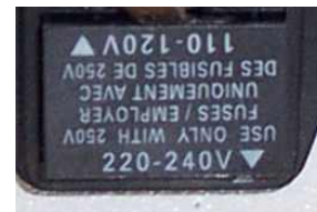
This is oriented for 220V operation
