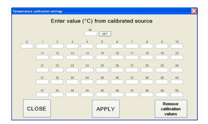
The temperature sensors are accurate to within  $\pm$  2°C over a range of 5°C - 60°C. To account for any Module-to-Module differences in temperature sensing capability, you can calibrate each sensor using the Temperature calibration settings screen. The values entered in the cells on this screen are used by the GPM software to determine the appropriate offsets to apply to each sensor to calibrate them to the temperature of your standard source.
