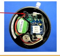
Make sure batteries are unplugged when not in use. If the batteries stay plugged into the modules when not in use it will greatly reduce their life and can even cause them to be unusable.
